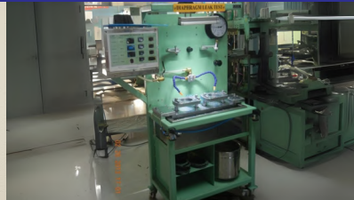
LEAK TESTING FIXTURE
